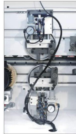
Flat scraping removes glue threads
